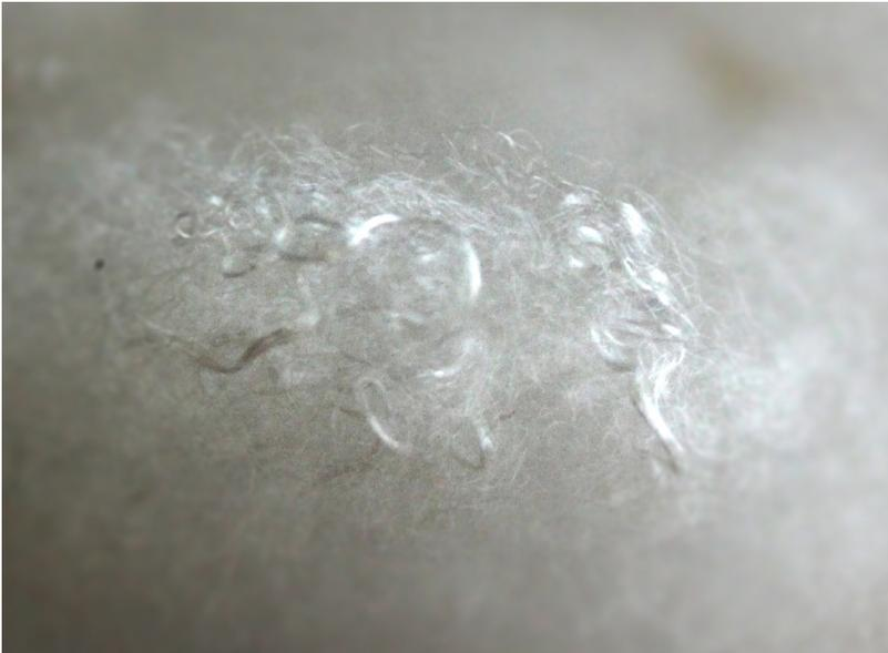
Close up of Ecodown® Fibers unique multi-shape structure.
